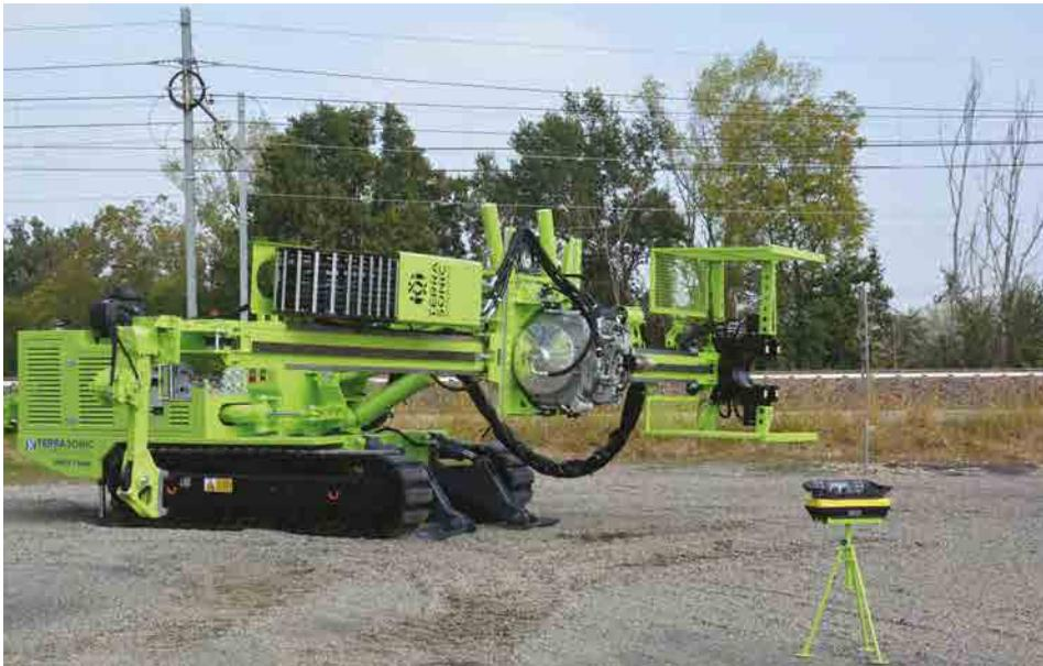
*The TSi 150CC-MM8 combines Massenza's MM8 drill rig with Terra Sonic International's 150 sonic drill head*
