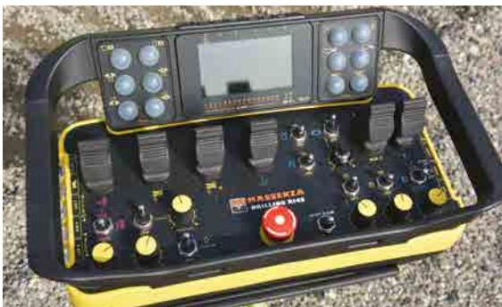
The remote control option of the existing Massenza MM8 is carried over to the new TSi 150CC-MM8
