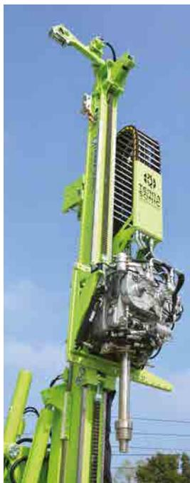
*The TSi 150 Sonic Oscillator provides an oscillator frequency of 0 to 150Hz, oscillator force up to 50,000lbs and a maximum torque of 4,677ft-lbs*
