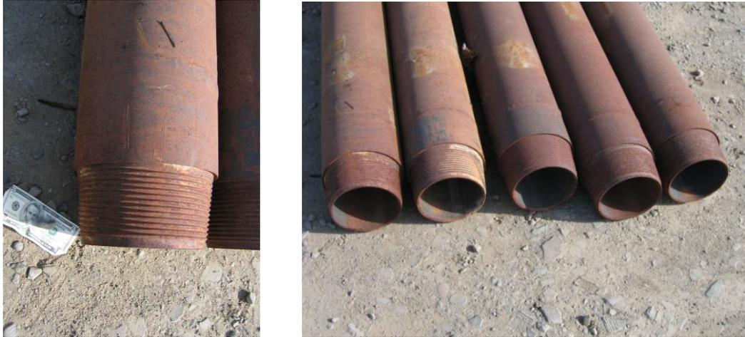
Figure 3.8. 9 inch outer diameter sonic drill pipe.
