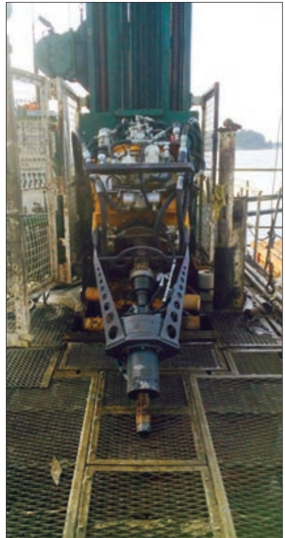
The Terra Sonic International sonic drill rig
