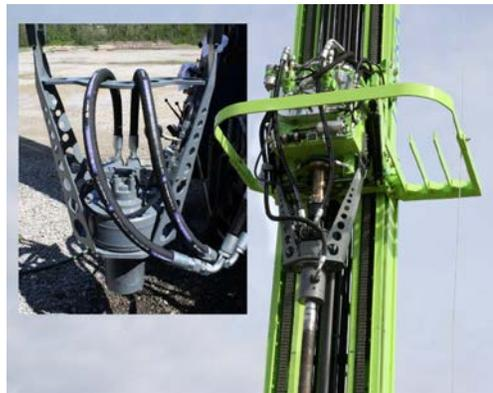
While Sonic Drilling can be used to extract hard rock cores, the Diamond Coring Option omits the use of the Sonic Head and Terra Sonic tooling, thereby increasing the efficiency of the hard rock coring process through the use of standard Diamond Coring tooling without wear and tear on the Sonic equipment. Terra Sonic provides 2-3/8" API female threads so that customers can adapt the tooling to their own specifications.
